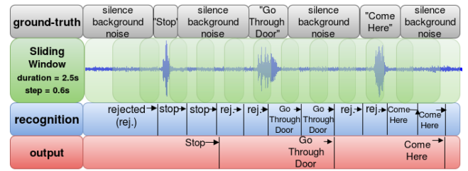
Figure 3: SPK node timeline: Sliding window based spoken command processing and recognition.
