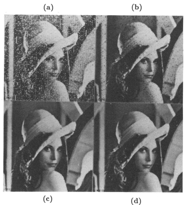
Figure 6. (a) An image f with salt-and-pepper noise (probability of occurrence of noisy samples is 0.1). (b) Opening f_B . (c) Open-closing (f_B)^B . (d) Median of f by the window W . ( B = \text{box} and W = \text{square} of Fig. 4.)
