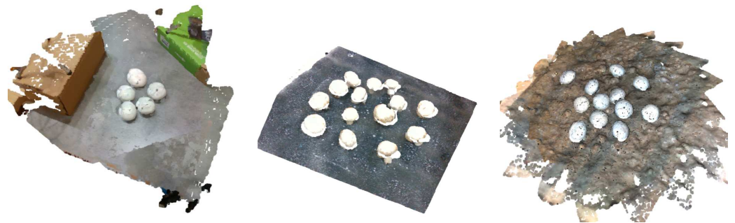
Figure 2. Three different settings of collected validation data: merged point cloud from 3 views using 3D printed mushrooms ( left ), merged point cloud from 2 views using real mushrooms ( center ) and merged point cloud from multiple views (18) using 3D printed mushrooms ( right ).
