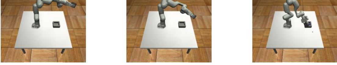
Fig. 3. Experimental Environment: We simulate the Franka Emika Panda robot arm pouring task within the TOTO framework. The goal is to transfer as many spheres as possible from the cup to the container.
