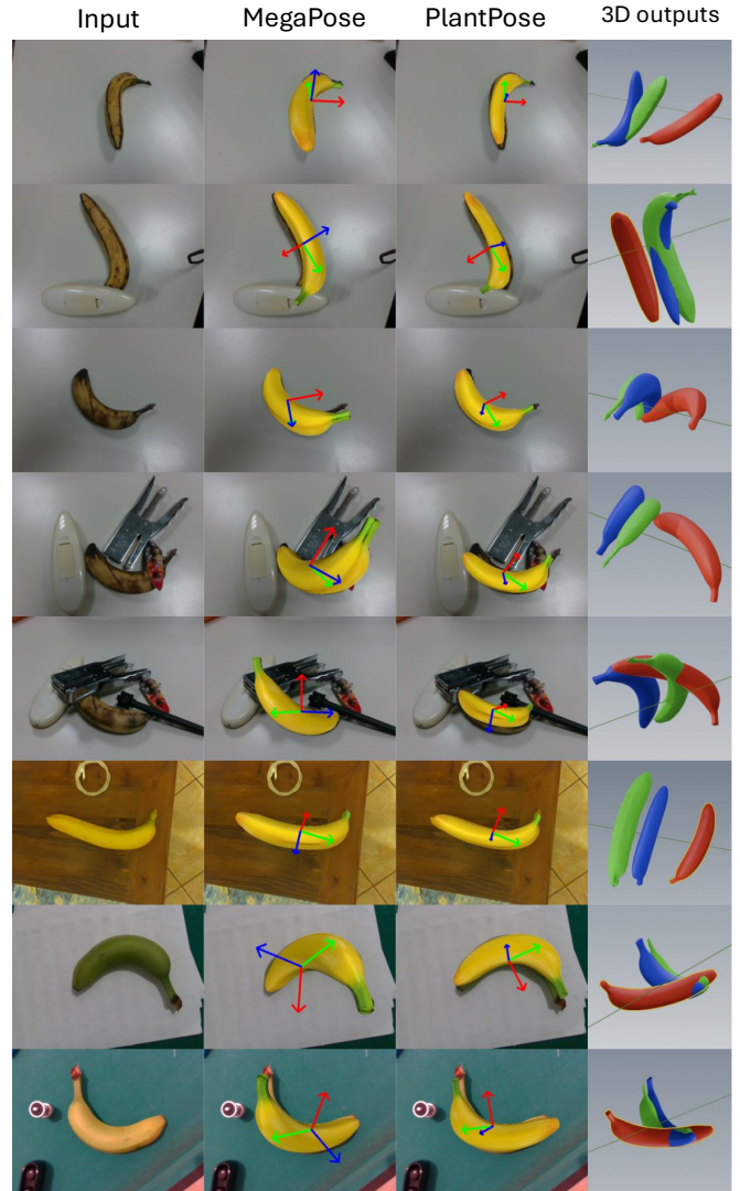
Fig. 3: Qualitative results on the banana test benchmark comparing MegaPose with PlantPose. The final column shows the predictions in 3D space (with a different angle to facilitate comparison): the green color denotes the ground truth mesh and 6D pose, blue is the result of PlantPose, and Red is the result of MegaPose.
