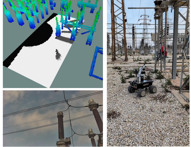
Fig. 1: Employment and testing of our proposed algorithm at a UHVC in Greece (right). Our mobile robot navigates to one of the optimally selected locations that exhibits a high visibility score for the electrical component under inspection (top left, Voltage Transformer shown in the green 3D bounding box), where our Viewpro Z10TIR RGB and thermal camera captures images for inspection and fault evaluation (bottom left).
