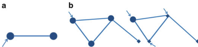
Fig. 3.3 Examples of structuring graphs. Arrows indicate roots. Large circular nodes denote buds. (a) The s-graph that corresponds to the simple neighborhood. Specifically, using this s-graph as a structuring element, the neighborhood of a node is the set of nodes that are adjacent to it. (b) A structuring graph and its reflection. The reflected s-graph has the same vertices and edges as the original s-graph but their bud and root sets are interchanged
