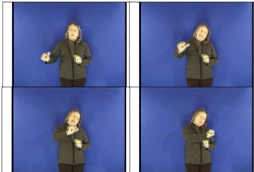
Fig.3. Segmentation and tracking of the image sequence from the sign video for the word “return” in GSL using computer vision techniques.
