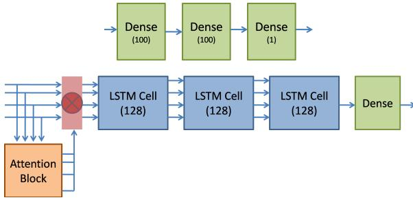
**Fig. 4.** A layer-level overview of the proposed chord switch detection (top) and candidate chord progression generator (bottom) networks.
