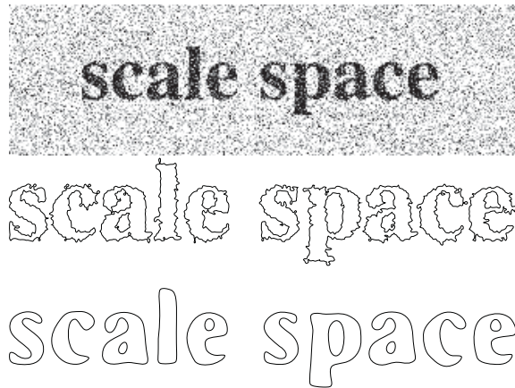
Fig. 1. Smoothing curves with the Affine Scale Space. Top: a text image corrupted by noise. Middle: thresholding the image reveals characters as irregular level lines. Bottom: the same level lines, smoothed with the affine scale space. The smoothing process produces curves almost independent of the noise, which is a requirement for robust pattern recognition. Algorithm used follows the affine erosion introduced in [48]. -Experiment courtesy of Lionel Moisan-
