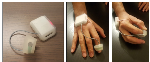
Figure 17: a) Motion tracking hand-wearable device. b) Thimble with the embedded pressure sensor for activation).
