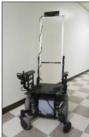
Fig. 1. A commercial electric power wheelchair with the Kinect 2 sensor mounted above the backrest, ensuring a wide field of view.
