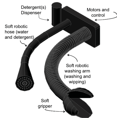
Fig. 1. Concept of the two robotic devices: (i) robotic hose and (i) robotic washing arm. The length of the robotic arm can vary depending the shower space and the ergonomic design. The concept is modular, self contained and easily interfaced with a conventional tab shower infrastructure.
