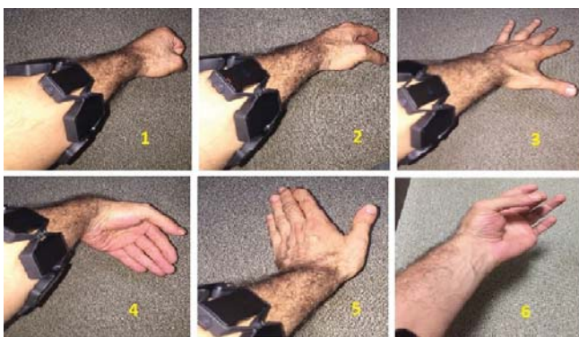
Figure 5. MYO armband and hand gestures, 1-Fist, 2-Hand relax, 3-Fingers spread, 4-Wave in, 5-Wave out, 6-Double tap conclusion
