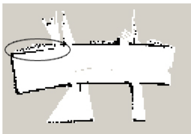
Figure 7. Occupancy Grid generated by the Dynamic ML-SLAM
