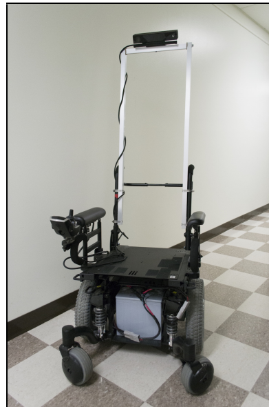
Fig. 1. A commercial electric power wheelchair with the Kinect 2 sensor mounted above the backrest, ensuring a wide field of view.
