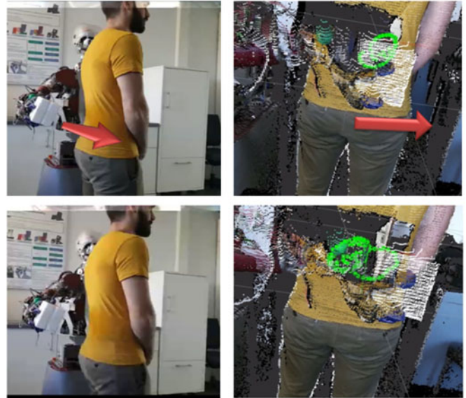
Fig. 10. Scenario III : ARMAR-III is wiping a male subject’s back region. The subject is moving to the right and the robot follows the motion. Left : Side camera view of the subject performing a translation to the right. Right : Zoomed Point cloud view of the experiment highlighting the adaptation of the wiping motion (green trajectory) to the movement of the subject. Safe distance is kept between the back and ARMAR-III’s end-effector.
