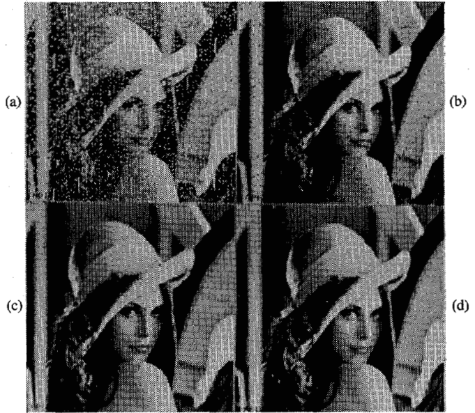
Fig. 1. (a) A 256 \times 256 -pixel (8-bit/pixel) graytone image f corrupted with salt-and-pepper noise; SNR = 15.1 dB. (Probability of occurrence of noisy samples is 0.1.) (b) Opening f_B of f by a 2 \times 2 -pixel square set B ; SNR = 19.5 dB. (c) Open-closing (f_B)^B ; SNR = 25.8 dB. (d) Median of f by a 3 \times 3 -pixel window; SNR = 29.1 dB. (The SNR's were computed by 20 \log_{10} (255/e_{\text{rms}}) , where e_{\text{rms}} was the rms-value of the difference between the original and the noisy or restored images.)
