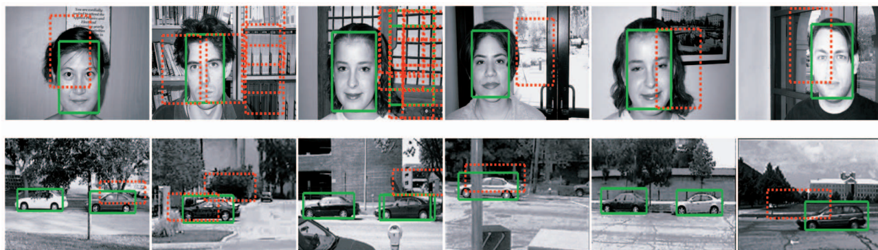
Fig. 12. Sample detection results on the data sets in [1], [14]. The locations proposed by a bottom-up detection system are used to initialize an EM loop, which brings in additional information from segmentation and the AAM parameters. Based on these, the initial hypotheses are either pruned (red dashed boxes) or validated (green boxes).
