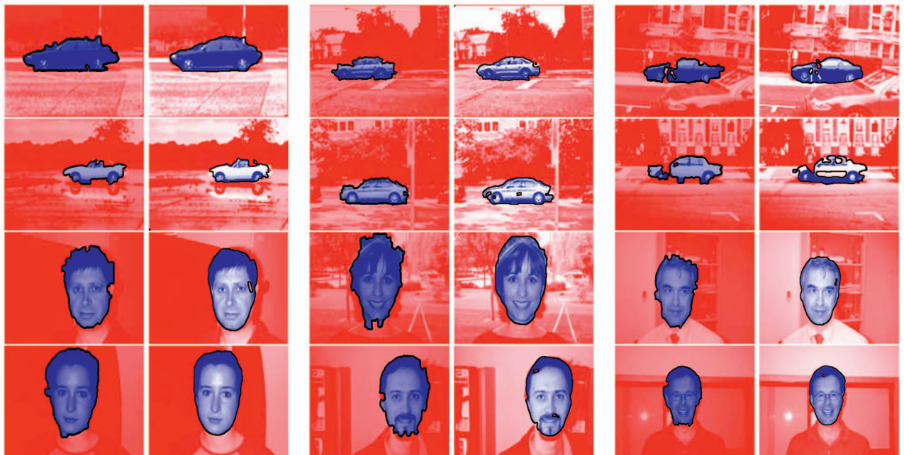
Fig. 7. Top-down segmentations of car and face images using (left) fragment-based and (right) curve evolution-based segmentation. For display, all background hypotheses are merged in a single region. For the fragment-based segmentation, we threshold the E-step results at a fixed value. We observe that the curve evolution-based results provide smoother segmentations, which accurately localize object borders.
