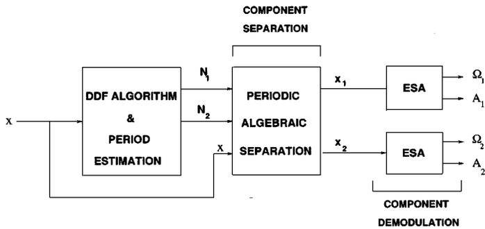
Fig. 1. Block diagram of the PASSED algorithm.
