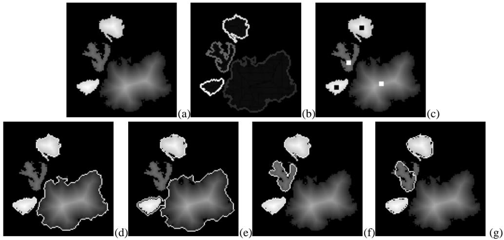
**Fig. 2.** (a) Synthetic image  $f$  (b) Gradient  $\|\nabla f\|$  (c) Markers (d) Vol. Flooding of  $f$  (e) Vol. Flooding  $\|\nabla f\|$  (f) Height Flooding of  $f$  (g) Height Flooding of  $\|\nabla f\|$ .
