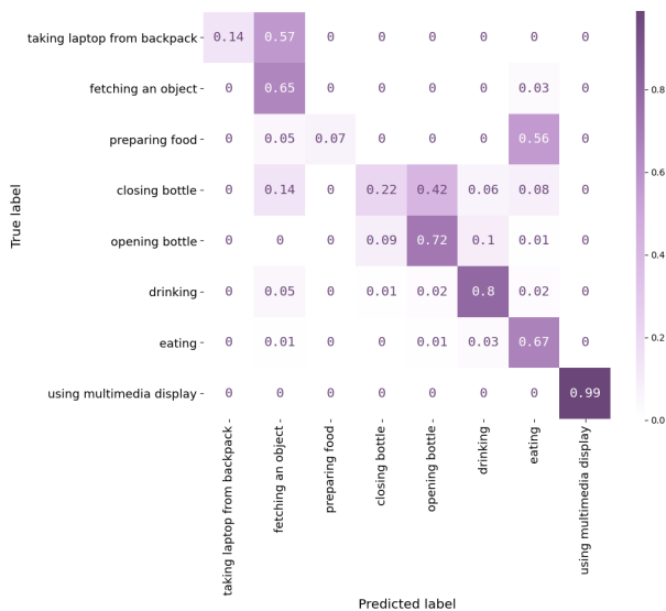
Figure 5: Subset of the normalized Confusion Matrix for the proposed model, i.e. early-fused 1/1/0+ TSM architecture.
